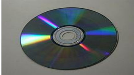
Figure(2.1)A CD-RW (CD), Chalcogenide forms glass the basis of rewritable CD and DVD solid-state memory technology
