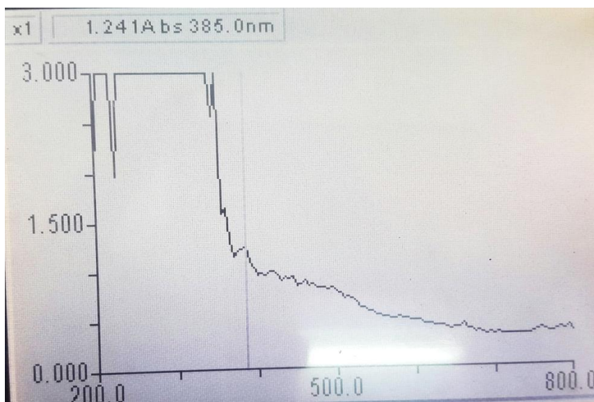
Figure (4.2)absorption of brown glass [ \lambda_{\max} = 385.0 nm]
