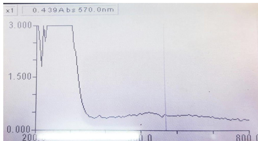
Figure (4.4) absorption of white glass [ \lambda_{\max}=570.0 nm]
