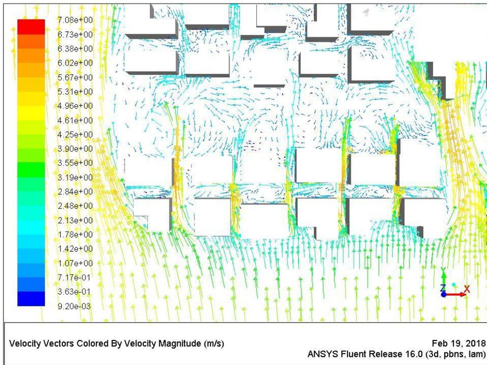
Figure 7.55 Wind pattern around buildings at a height of 4.5m [Author]
