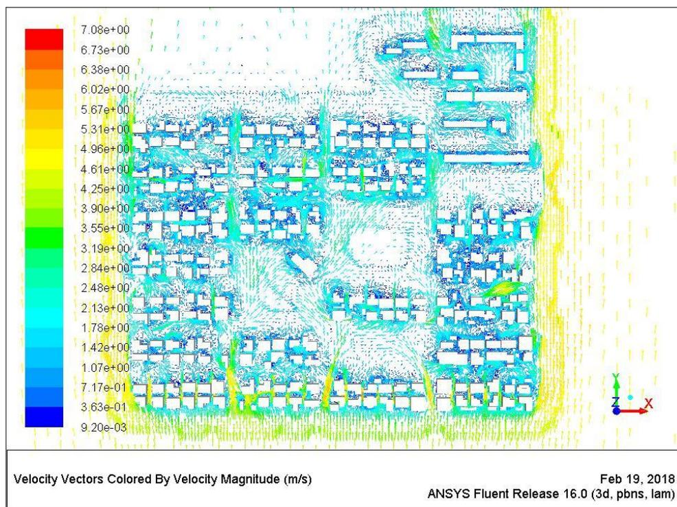
Figure 7.50 Wind pattern around buildings at a height of 1.5m [Author]
