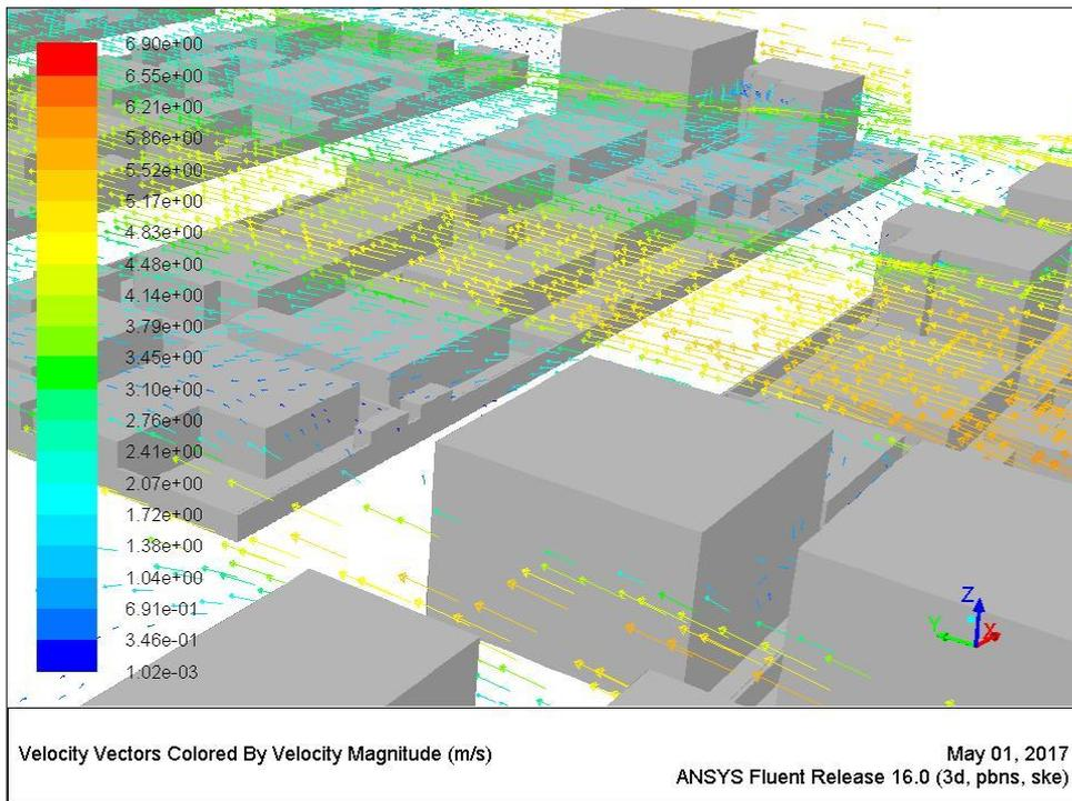
Figure 7.44 Wind path lines around buildings at height 10.5 m. [Author]
