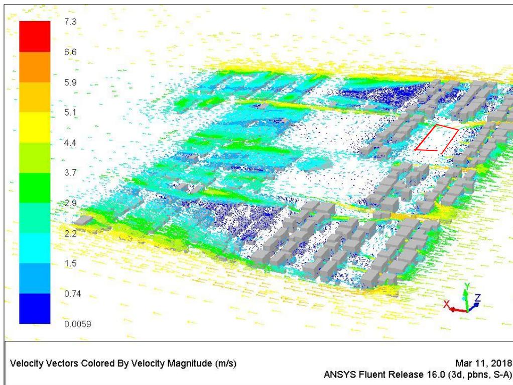
Figure 7.70 Wind pattern around buildings at a height of 7.5m [Author]
