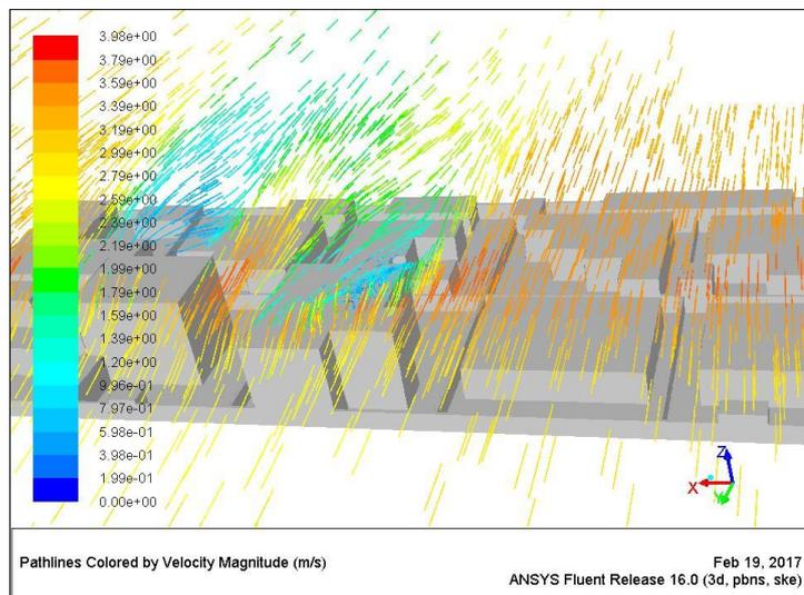
Figure 7.31 shows the wind pattern around buildings at a height of 10.5 m. [Author].
