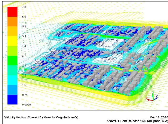
Figure 7.66 Wind pattern around buildings at a height of 1.5m [Author]
