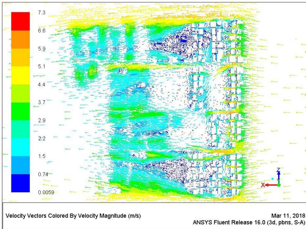
Figure 7.71 Wind pattern around buildings at a height of 7.5m [Author]
