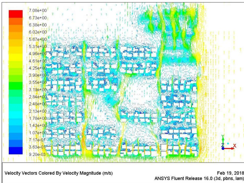
Figure 7.56 Wind pattern around buildings at a height of 7.5m [Author]
