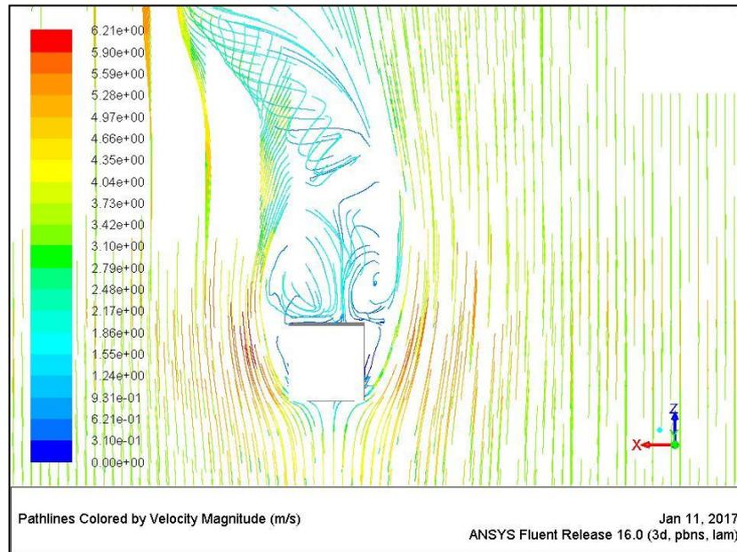
Figure 7.11 Speed and direction of the wind around the building (mesh 0.5). [Author]
