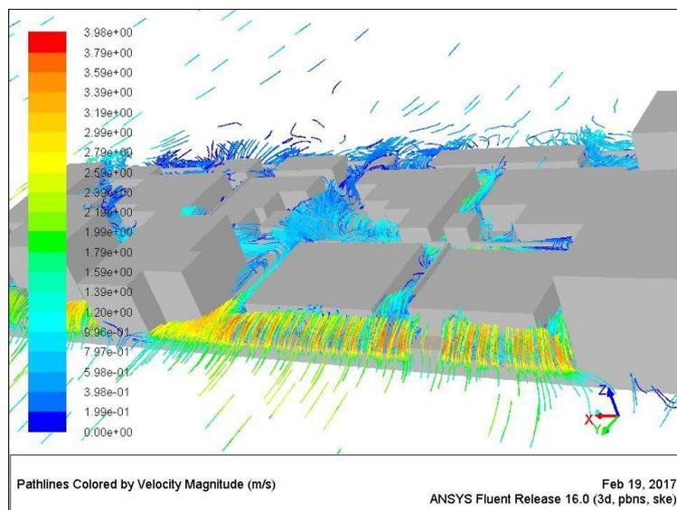
Figure7.25 wind pattern around buildings at 1.5 m.
