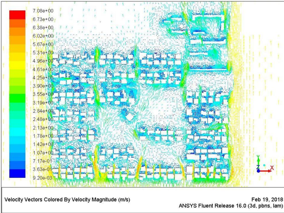
Figure 7.53 Wind pattern around buildings at a height of 4.5m [Author]
