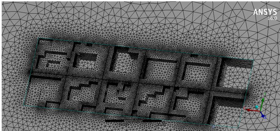
Figure7.21 2D shows Tetrahedran mesh generated by Ansys 16 software. [Author].
