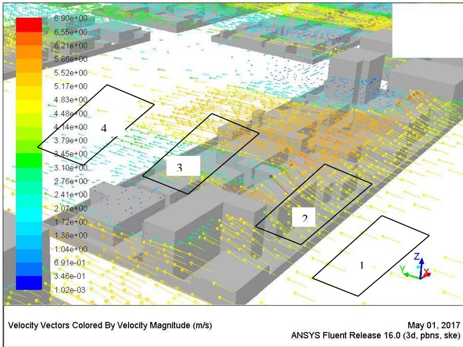
Figure 7.43. Wind path lines around buildings at height 10.5 m. [Author].
