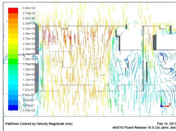
Figure 7.28 Wind pattern around buildings at a height of 7.5 m. [Author].
