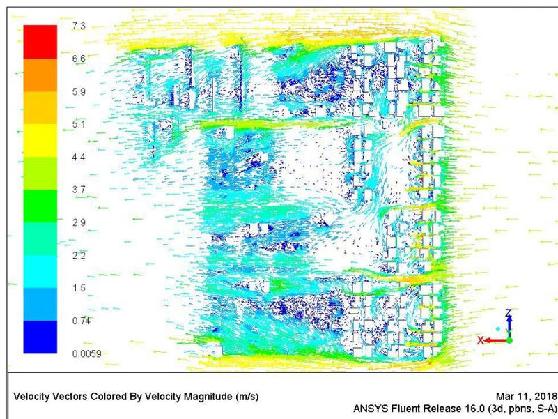
Figure 7.69 Wind pattern around buildings at a height of 4.5m [Author]
