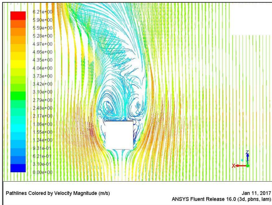
Figure 7.12 speed and direction of the wind around the building (mesh 0.1). [Author]
