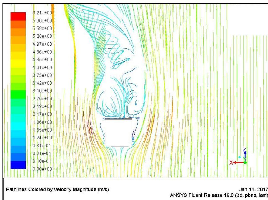
Figure 7.9 Wind pattern around the building (speed and direction) [Author]
