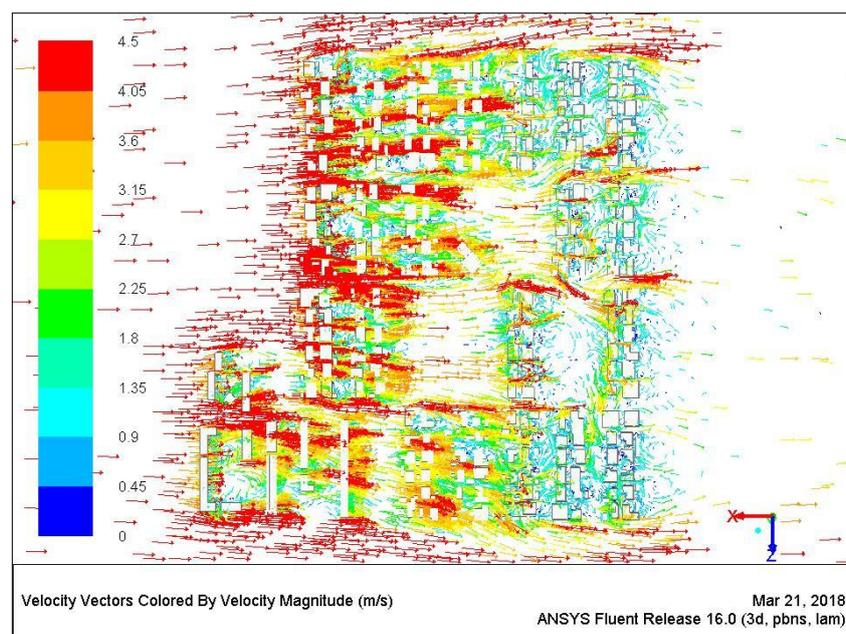
Figure 7.78 Wind pattern around buildings at a height of 7.5m [Author]
