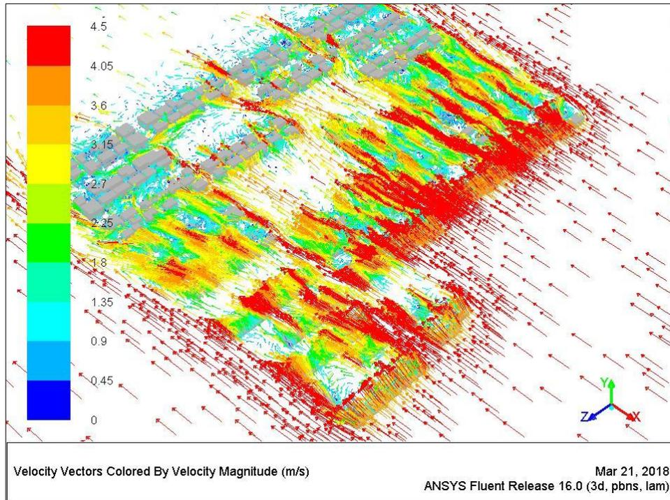
Figure 7.79 Wind pattern around buildings at a height of 7.5m [Author]
