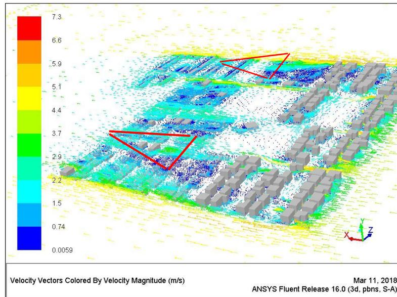
Figure 7.68 Wind pattern around buildings at a height of 4.5m [Author]
