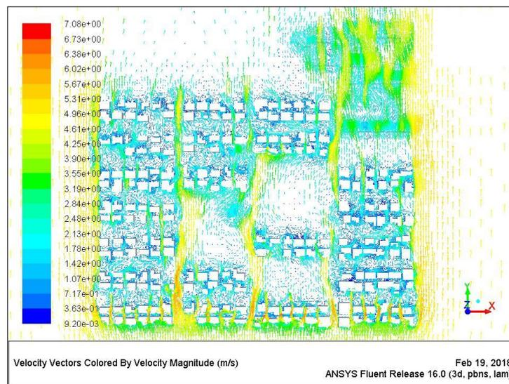
Figure 7.59 Wind pattern around buildings at a height of 10.5m [Author]
