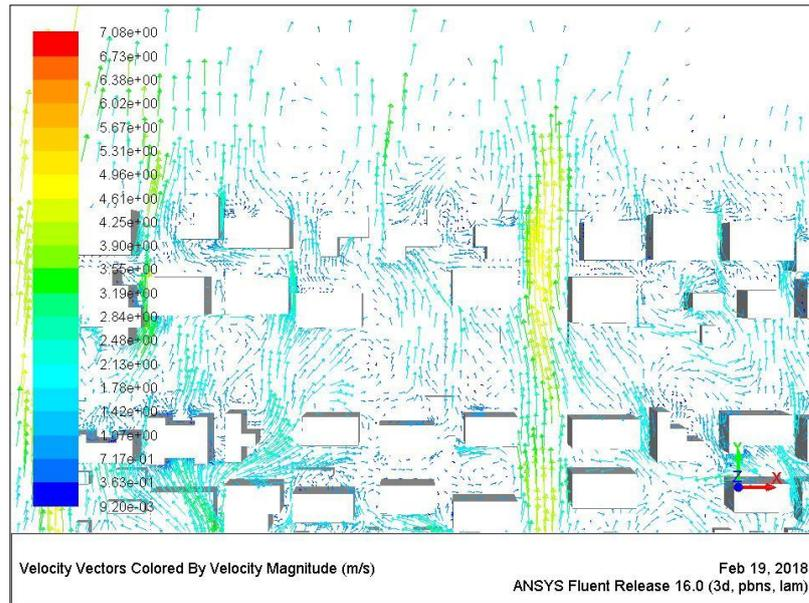
Figure 7.61 Wind pattern around buildings at a height of 10.5m [Author]
