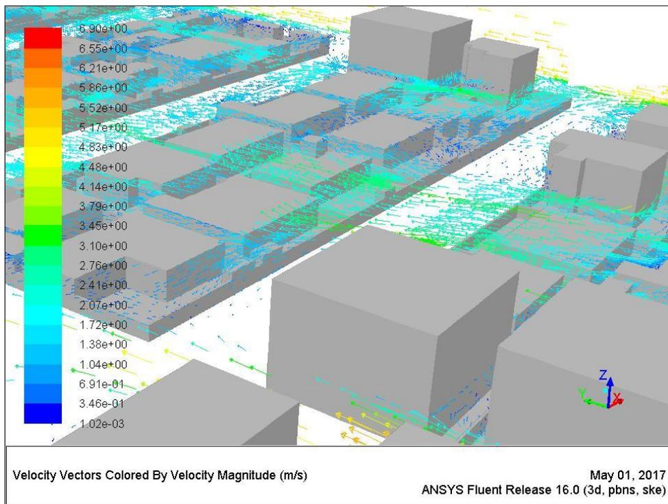
Figure 7-40 Wind path lines and speed around buildings at 4.5m. [Author]
