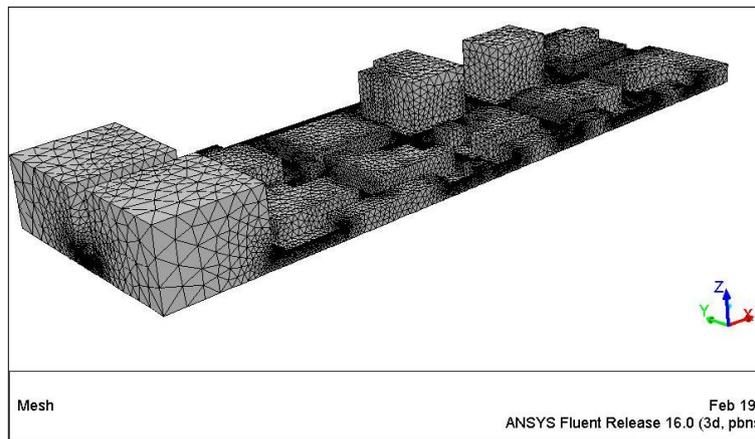
Figure7.19 3D Tetrahedran mesh generated by Ansys 16 software. [Author].
