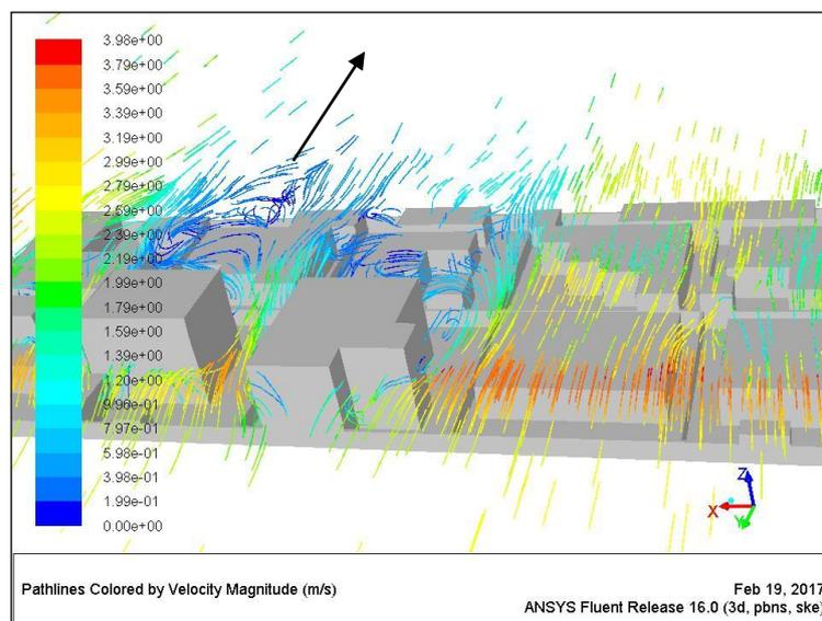
Figure7.27 Wind pattern around buildings at a height of 4.5
