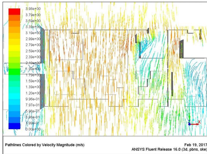
Figure 7.30 Wind pattern around buildings at a height of 10.5 m. [Author].
