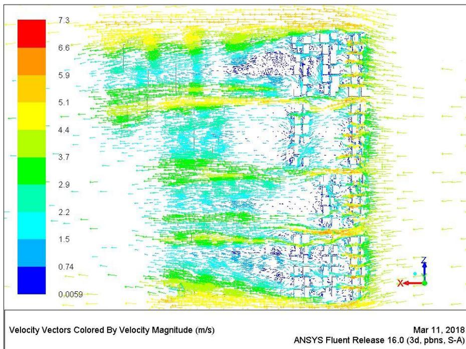
Figure 7.73 Wind pattern around buildings at a height of 10.5m [Author]
