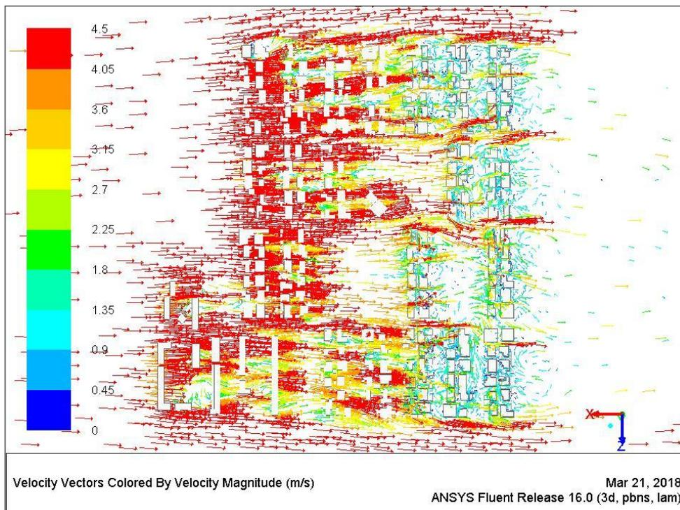
Figure 7.80 Wind pattern around buildings at a height of 10.5m [Author]
