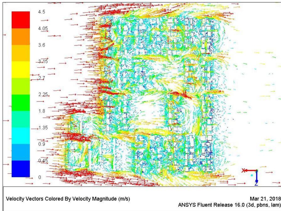
Figure 7.75 Wind pattern around buildings at a height of 1.5m [Author]
