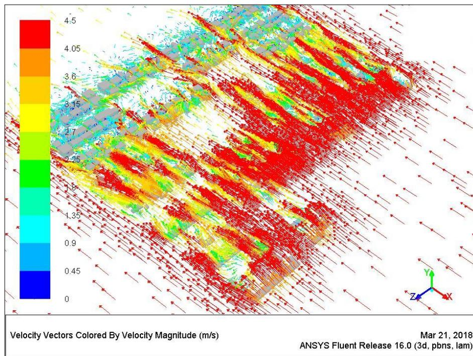
Figure 7.81 Wind pattern around buildings at a height of 10.5m [Author]
