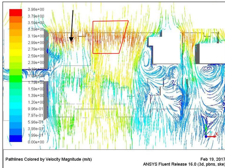
Figure7.26 Wind pattern around buildings at a height of 4.5 m.
