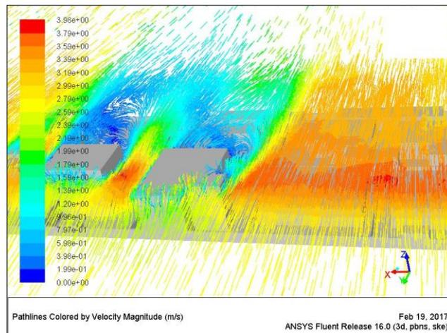
Figure 7.29 Wind pattern around buildings at a height of 7.5 m. [Author].
