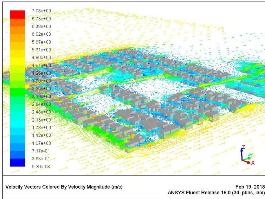
Figure 7.57 Wind pattern around buildings at a height of 7.5m [Author]
