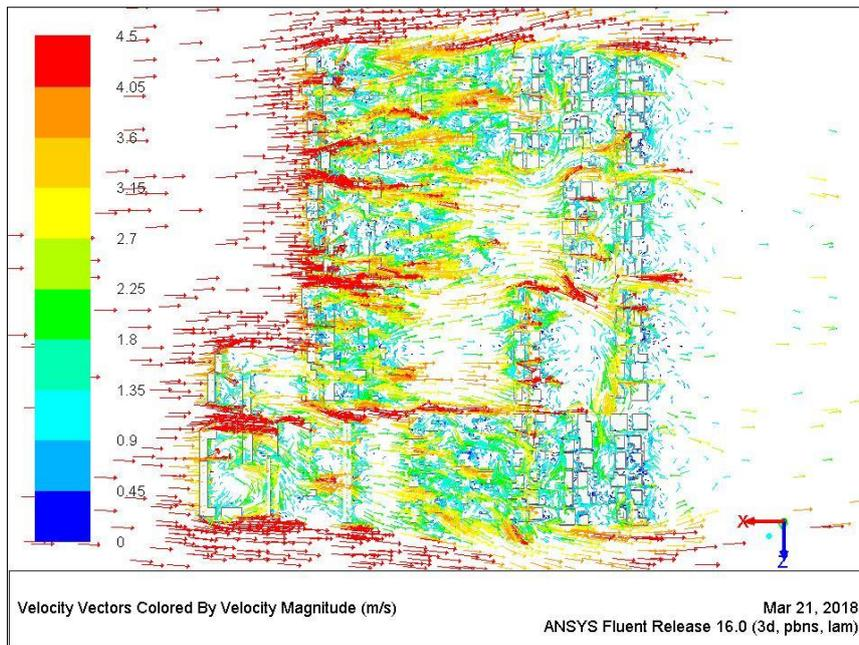
Figure 7.76 Wind pattern around buildings at a height of 4.5m [Author]
