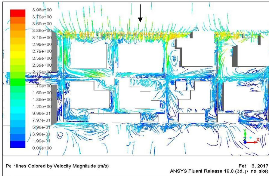
Figure7.22 Wind pattern around buildings at 1m.
