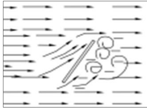
Figure (3.10) Permanency of the wind flow Figure (3.11) Pressure zone around barrier Figure (3.10& 3.11): Wind pattern around barriers. [Darcin, 2010].
