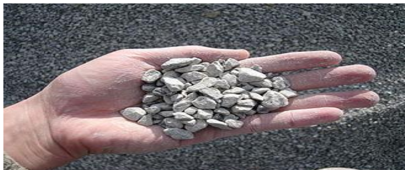
Figure 2-1: Crushed stone aggregate
