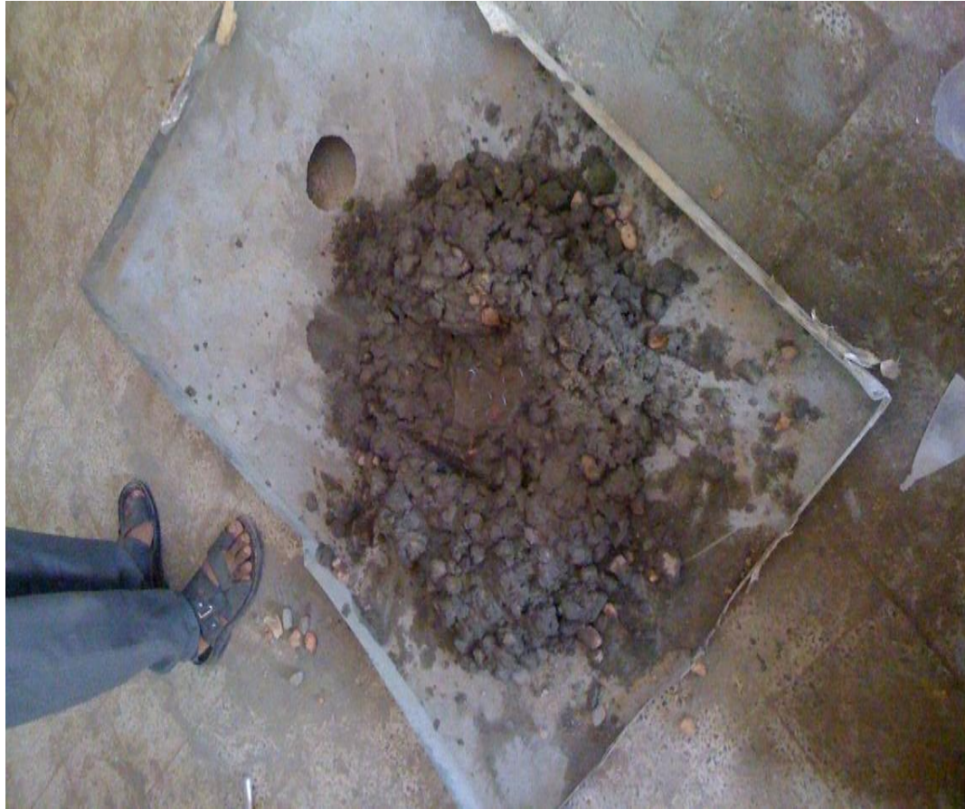
The concrete mix M (0) without add Superplasticizer admixture
