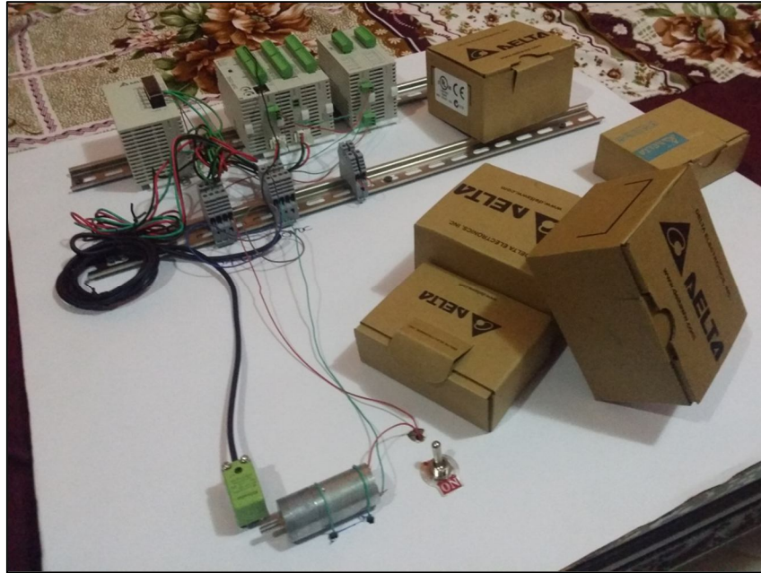
Figure 4-23: the model after installing DC motor and its switch and speed sensor.
