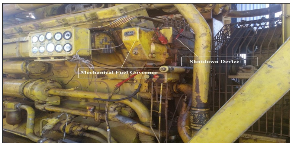
Figure 2-9: Mechanical fuel governor 1.Mechanical governor. 2. Shutdown device.(Jinan, 2005)
