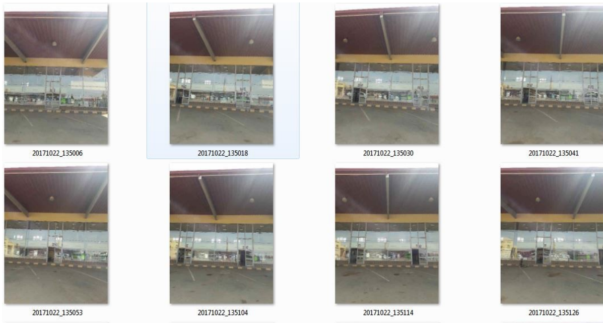
Figure (5.3): (B) a second set of overlapping photos It is important to note that the overlaps along the movement and perpendicular to it should be in a range of 80%. The higher the overlap ratio the better is the reconstruction of 3D point clouds.
