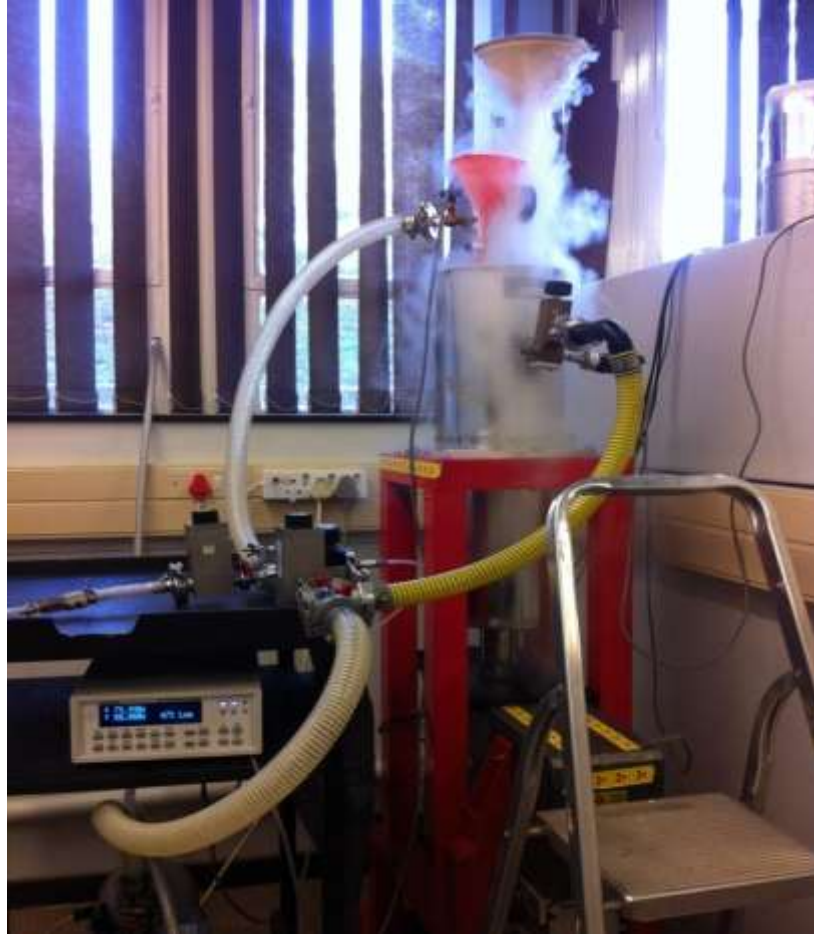
Figure 3.2. Mössbauer spectrometer cryostat, Condensed Matter Physics Laboratory, Westville Campus, South Africa.
