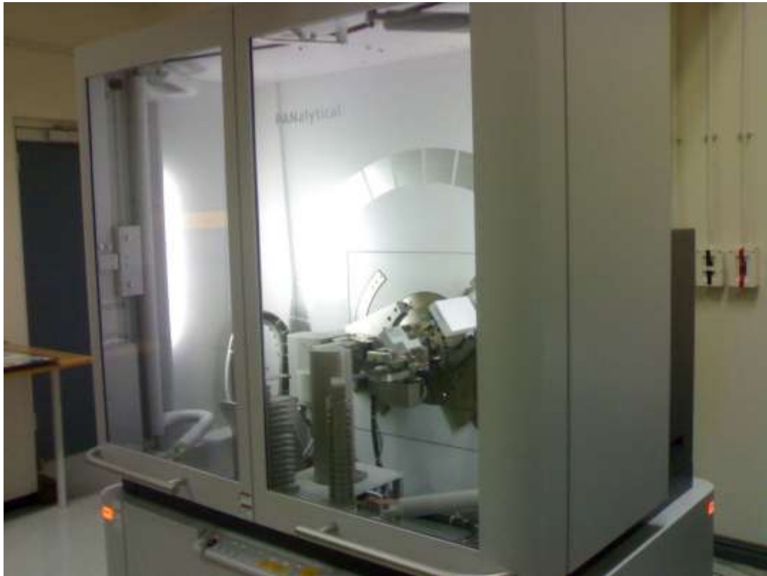
Figure 3.4. Empyrean PANalytical X-ray diffractometer cabinet, Geology Westville campus, University of KwaZulu-Natal, South Africa.
