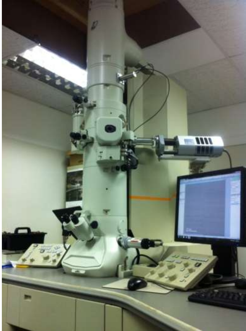
Figure 3.5. Joel-JEM-2100 high resolution transmission electron microscope, Westville campus, University of KwaZulu-Natal, South Africa.
