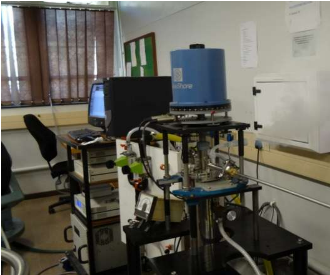
Figure 3.6. LakeShore model 735 vibrating sample magnetometer (VSM), Condensed Matter, University of KwaZulu-Natal, South Africa.
