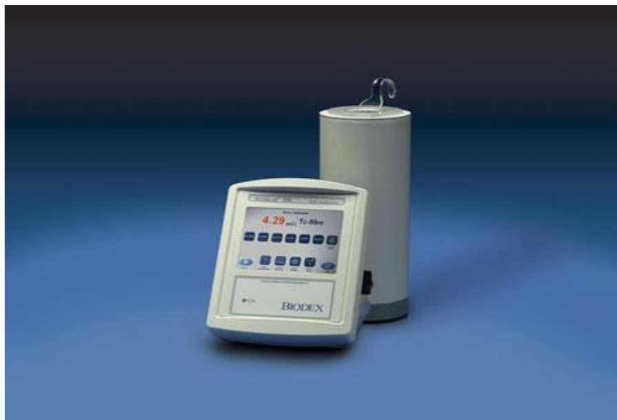
Figure 2.2 A radionuclide dose calibrator, Biodex model Atomlab 500. (Photo courtesy of Biodex Medical Systems, Inc.)
