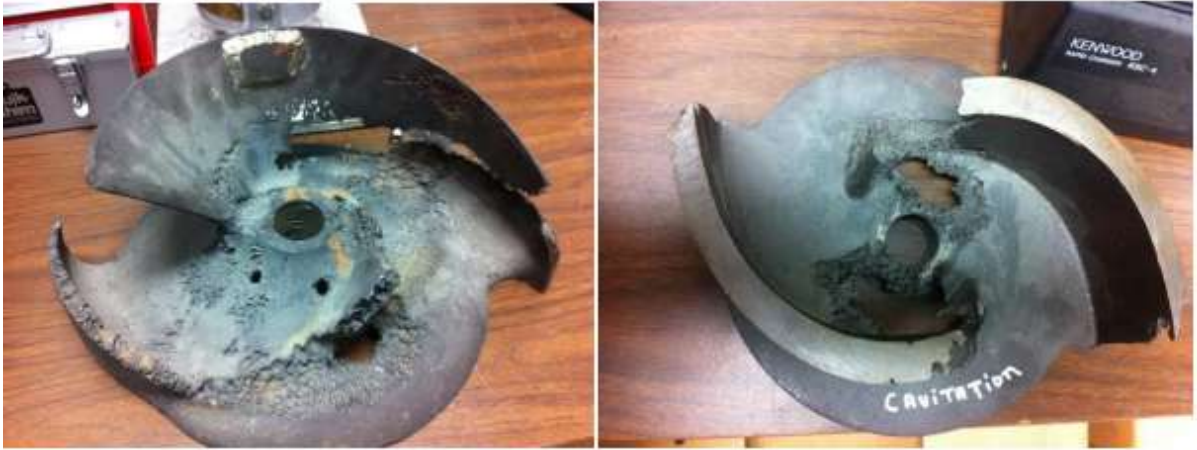
Figure (3.7) pumps cavitation
