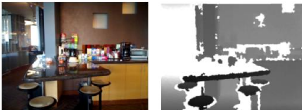
Fig 2.6 (left) RGB image and (right) depth information captured by an RGB-D camera. White pixels in the right image have no depth value, mostly due to occlusion, max distance, relative surface angle, or surface material. [6].
