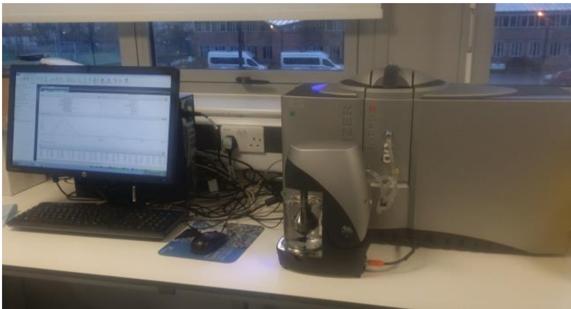
Figure.2.10. Mastersizer 3000, a laser diffraction particle size analyzer (Malvern Instruments)
