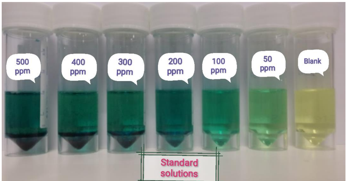
Figure.2.3. The blank, and standard solutions of standard Gallic acid
