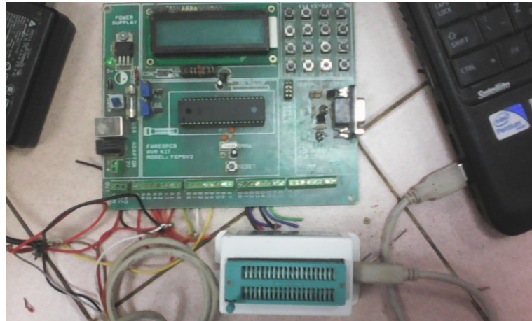
Figure-4 (a): The circuit used for humidity measurement collected by researcher
