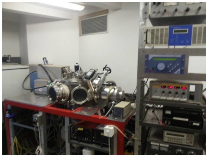
Figure.7 The sputter deposition system WARNING (Wits) of Technology Lab.
