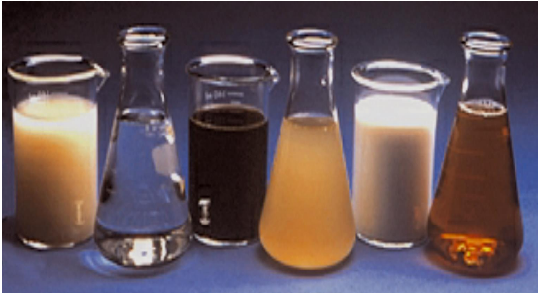
Figure 2-5: Liquid admixtures, from left to right: anti-washout admixture, shrinkage reducer, water reducer, foaming agent, corrosion inhibitor, and air-entraining admixture
