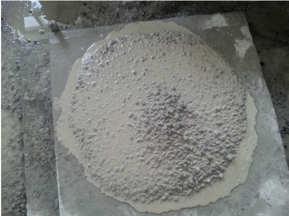
Figure 2-6: Flow test for segregated concrete
