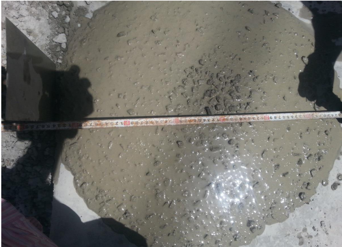
Figure 3-1: Concrete flow test
