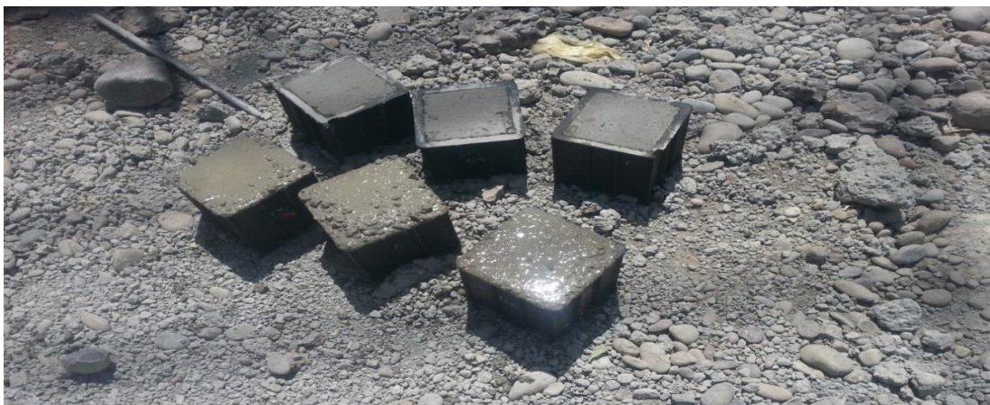
Figure 3-2: The cubes after fresh concrete process
