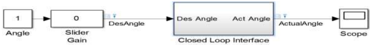
Figure 3.16: Simulink model (code) of host computer
