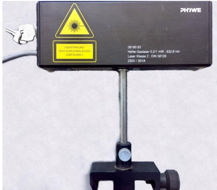
Fig. 3.2. He-Ne laser device.
