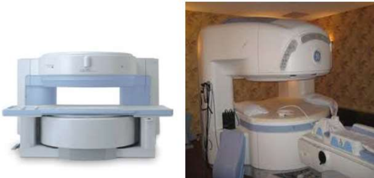
Figure 2-7 MRI Machine - Permanent Magnets
