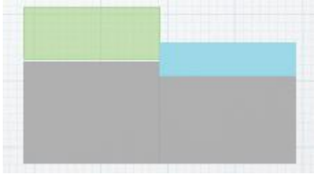
Figure 2.4 Grow a second oxide layer.
