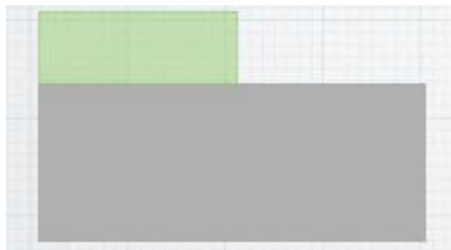
Figure 2.3 Grow an oxide layer.
