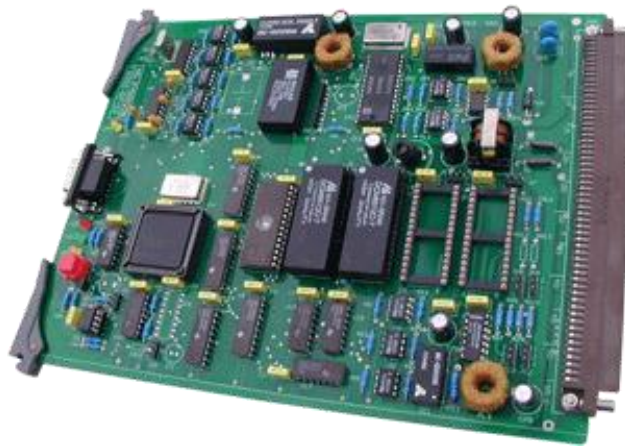
Figure 3.12: Communication and storage board
