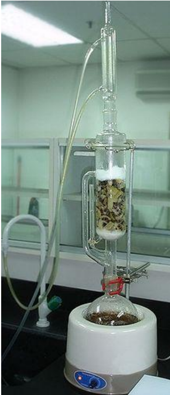
Soxhelt extractor apparatus
