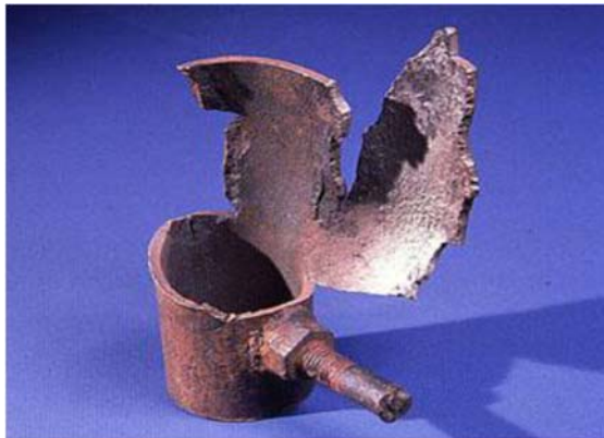
Figure 2.24: Failure caused Internal Corrosion-Hydrogen Damage.
