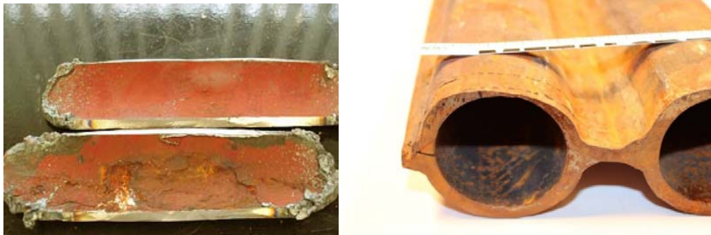
Figure 2.22: Failure caused by internal erosion.
