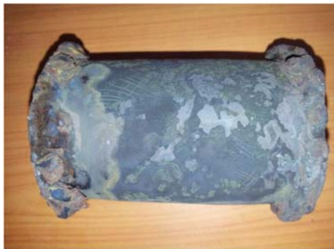
Figure 2.21: Failure caused Thermal fatigue.
