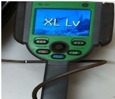
Figure 3.7: XL LV Bore scope (inspection device).
