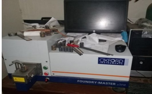
Figure 3.4: (ICP- OES) Chemical Composition Measurement.
