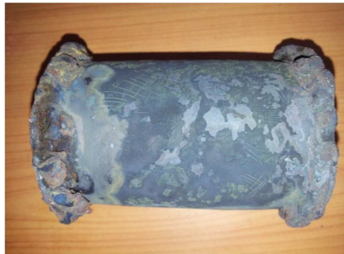
Figure 2.21: Failure caused Thermal fatigue.
