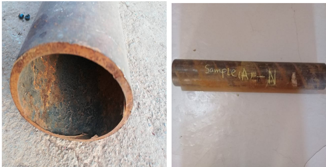
Figure3.1: New sample (Original), before test.
