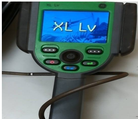
Figure 3.7: XL LV Bore scope (inspection device).
