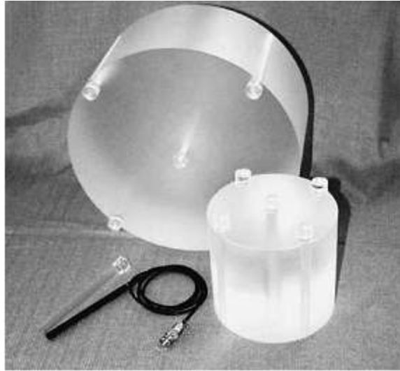
Figure (2.13) Cylindrical standard computed tomography (CT) dosimetry phantoms (16 cm and 32 cm in diameter) made from Perspex for representative measurements of the computed tomography dose index (CTDI) in regions of the head and the trunk, and a pencil-like detector for measurements of the dose-profile integral
