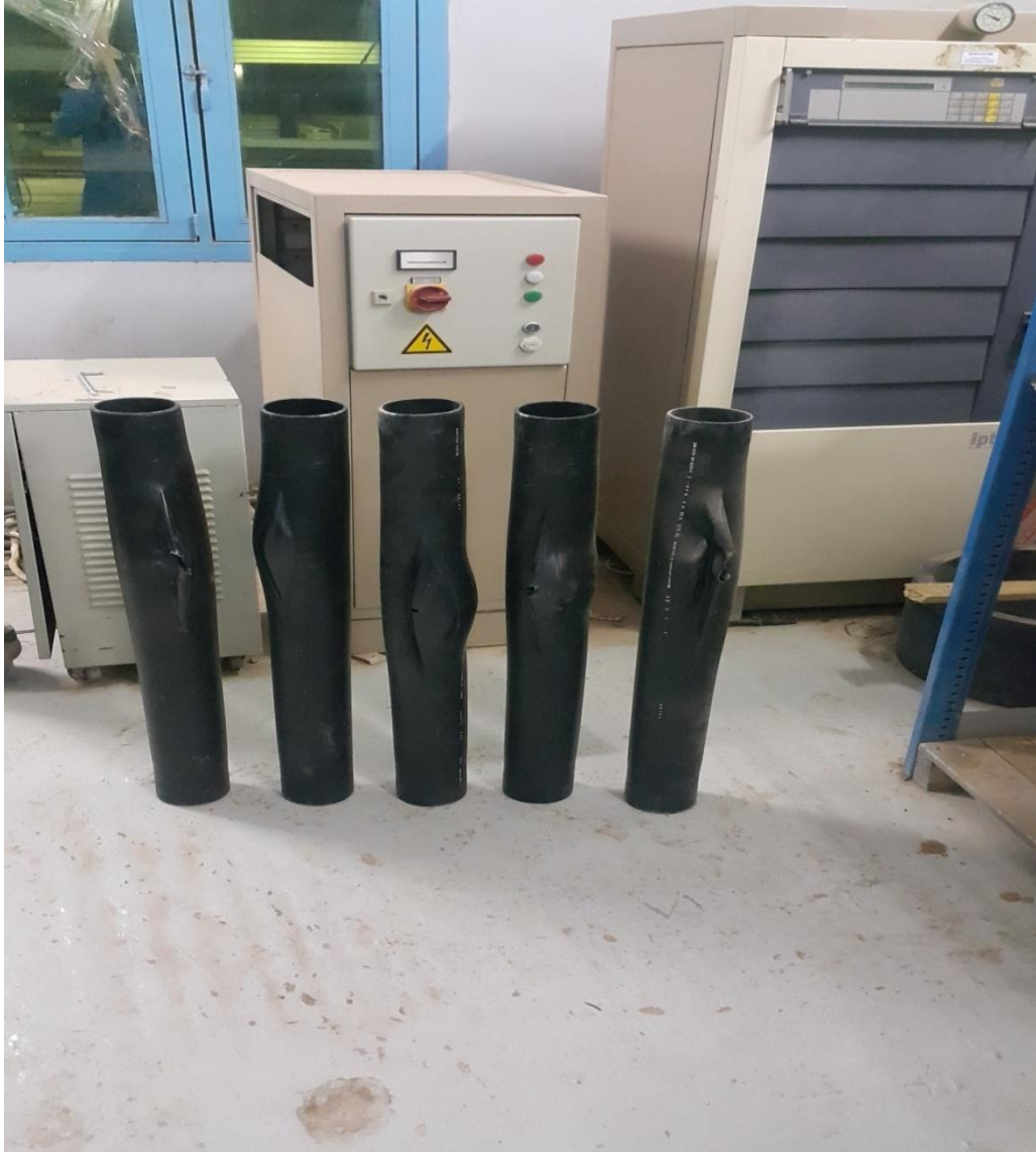
Fig (4.3): shape of specimen after failure.
