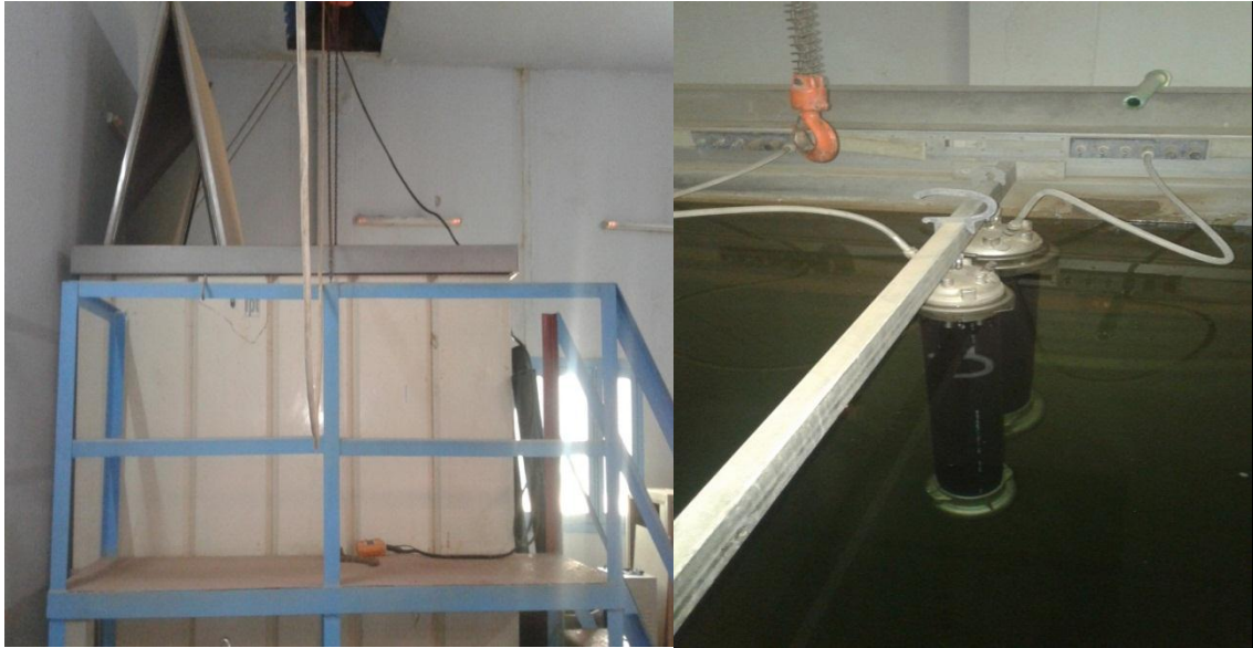
Fig (3.4): tank for hydrostatic pressure test
