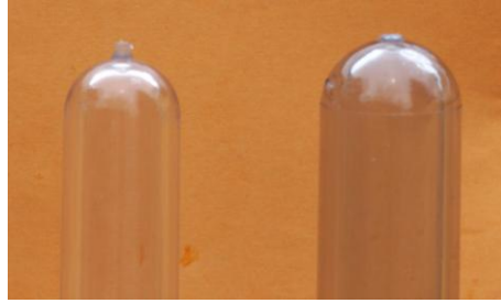
Figure 2.6 Typical difference in length of gate
