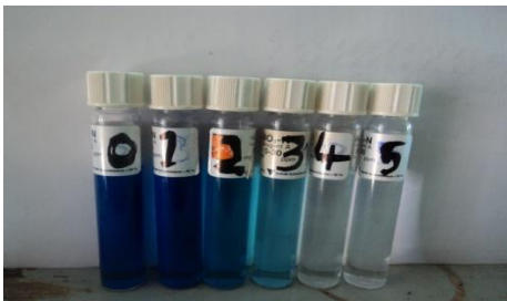
Fig. (A-1): Change methylene blue colour (a) at first hour (b) after five hour (c) treatment by using pure \text{TiO}_2 (d) treatment by using \text{TiO}_2 sol-gel
