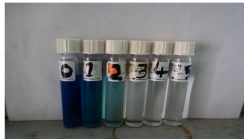
Fig. (A-1): Change methylene blue colour (a) at first hour (b) after five hour (c) treatment by using pure \text{TiO}_2 (d) treatment by using \text{TiO}_2 sol-gel
