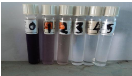
Fig. (A-2): Change tubantoin blue colour (a) at first hour (b) after five hour (c) treatment by using pure \text{TiO}_2 (d) treatment by using \text{TiO}_2 sol-gel
