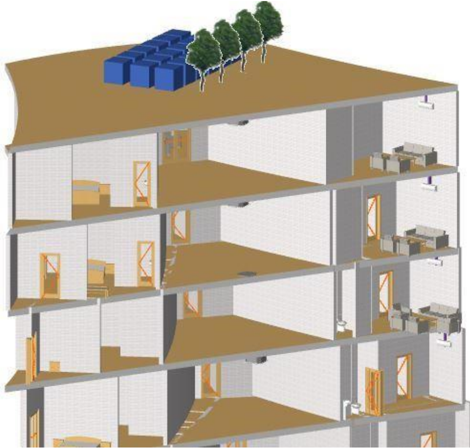
Vrv air conditioning system
