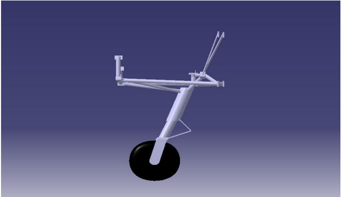
Figure 16 mount and nose landing gear for new engine from side view
