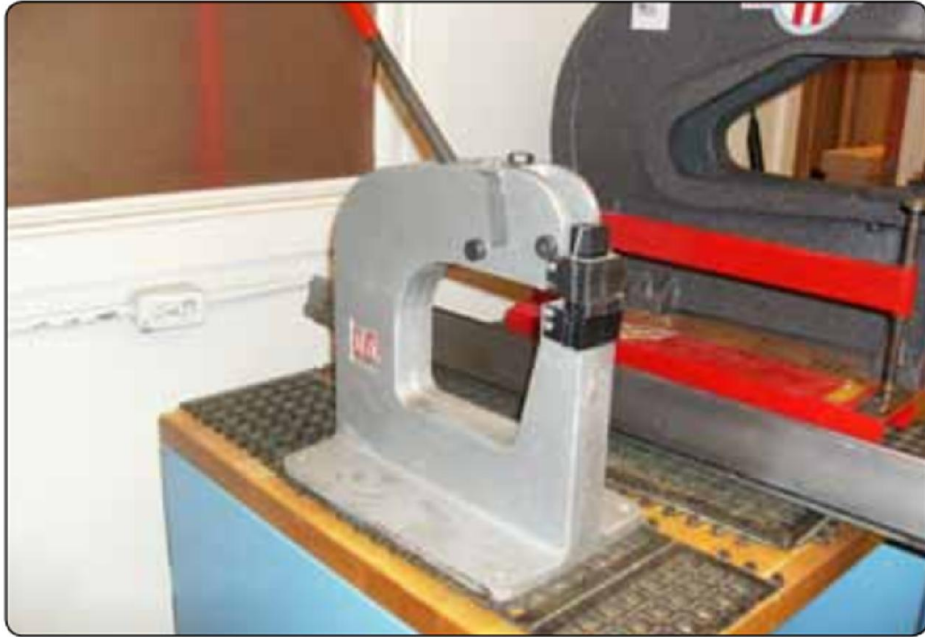
Figure 3-2 Stretching &shrinking machine
