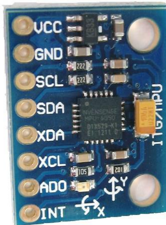
Figure 19: MPU6050 IMU used in our quadcopter
