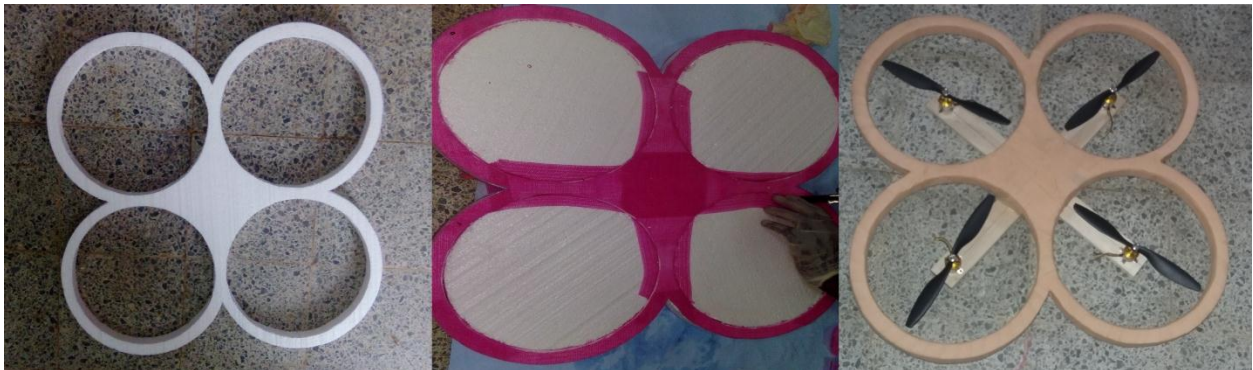
Figure 16: Plastic foam frame incase in fiber glass
