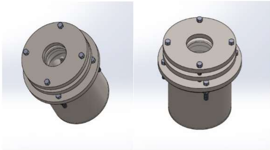
Figure 3. 5 show 3D model of the reactor which was created by SolidWorks
