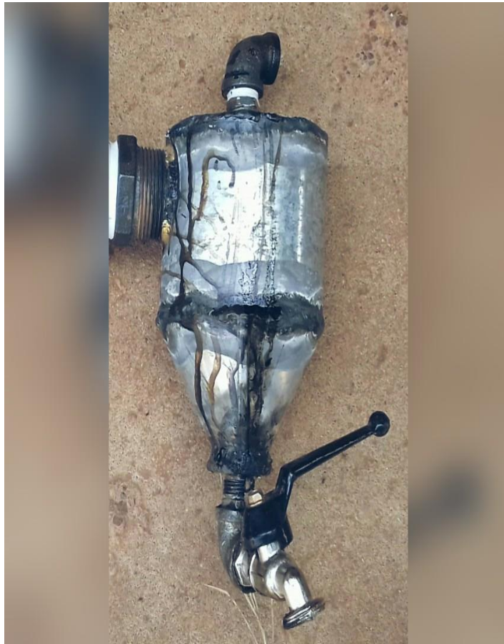
Figure 3.4 show the designed separator.
