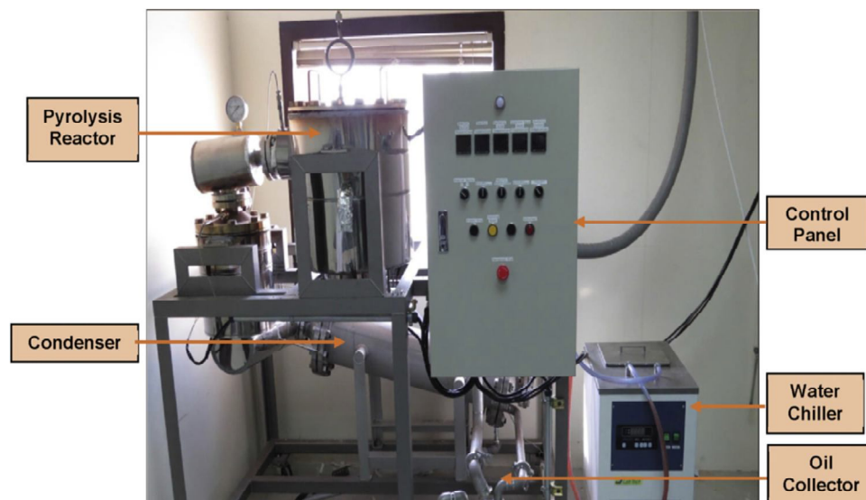
Figure 2.17: Small pilot scale Batch Pyrolyzer Reactor [23].
