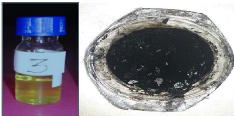
Figure 2.21: Condensed oil and char obtained [48].
