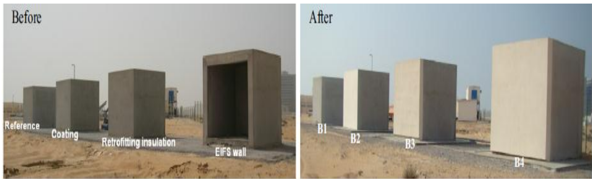
Figure2 1 four cubical calorimeter at site with different south wall configuration
