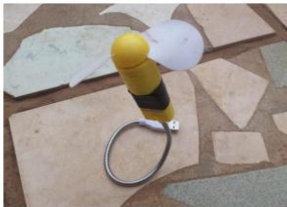
Figure (3.7): A fan using for increasing the rate of heat transfer
