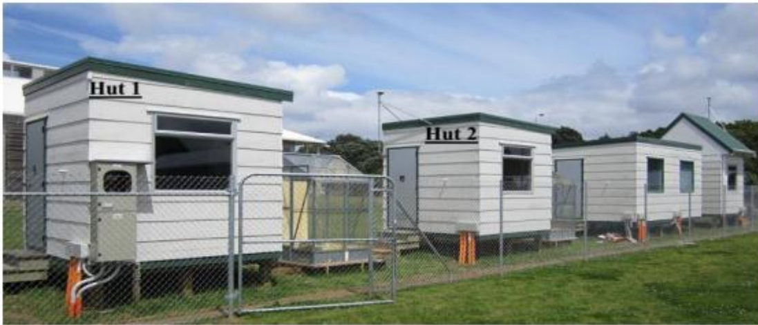
Figure (2.9): Wood-framed test huts built for PCM testing on the Tamaki Campus , University of Auckland, New Zealand [49, 50].
