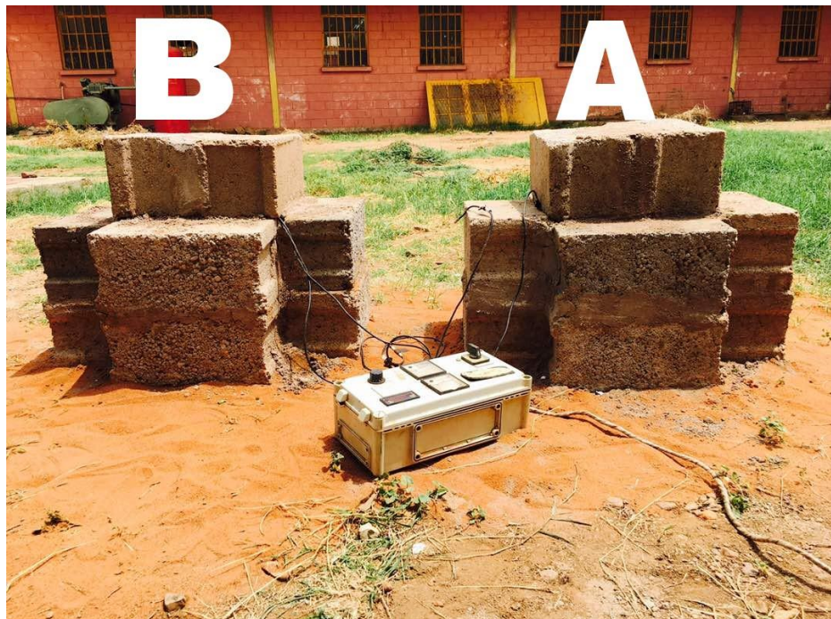
Figure (3.2): Two small-models, model (A) without PCM and model (B) with PCM
