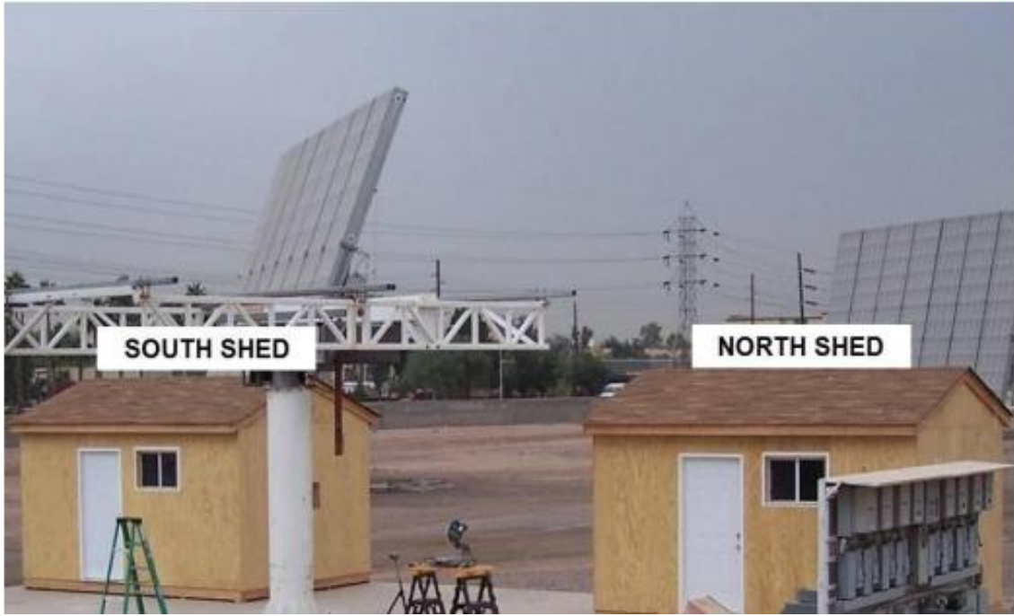
Figure (2.4) Experimental Setup of South (non BioPCM) Shed and North (BioPCM) shed.
