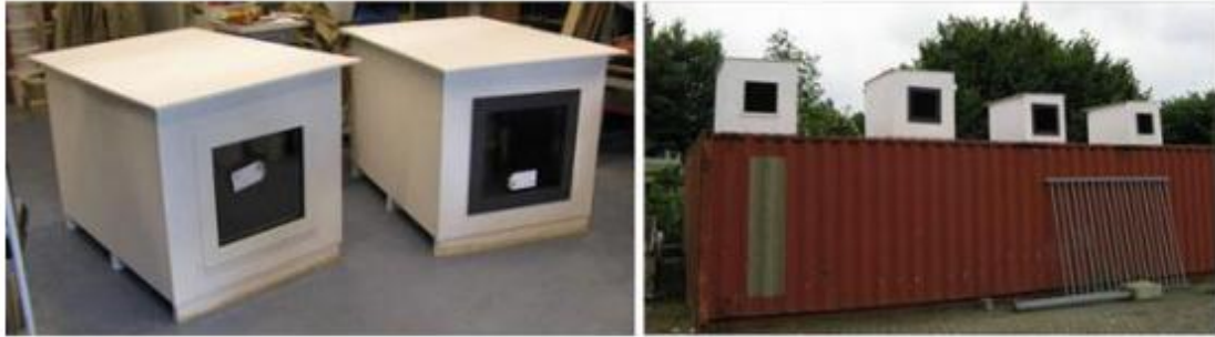
Figure (2.26): University of Twente test boxes for PCM floor testing [60, 61].
