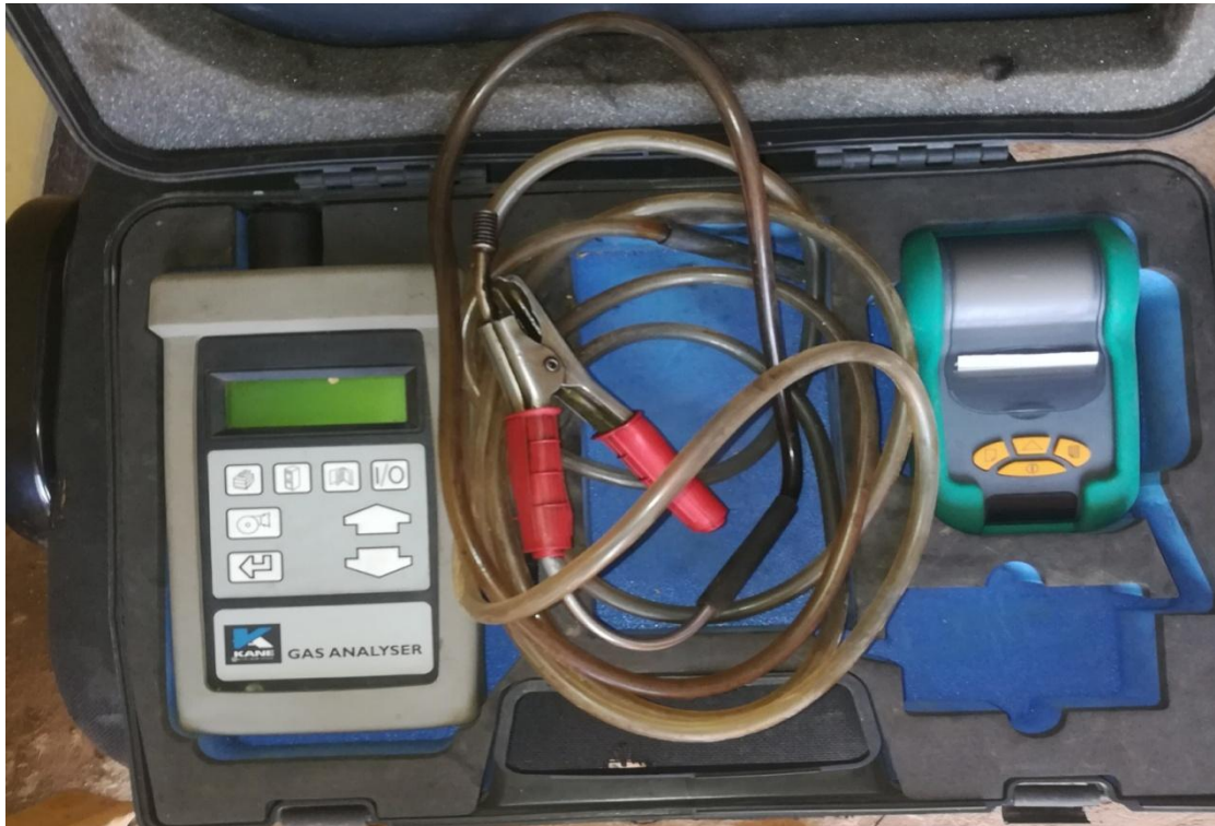
Figure (3.4) shows gas analyzer
