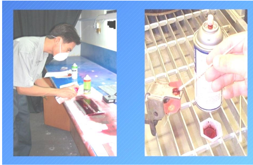
Fig. (3. 5) Penetrated Inspection
