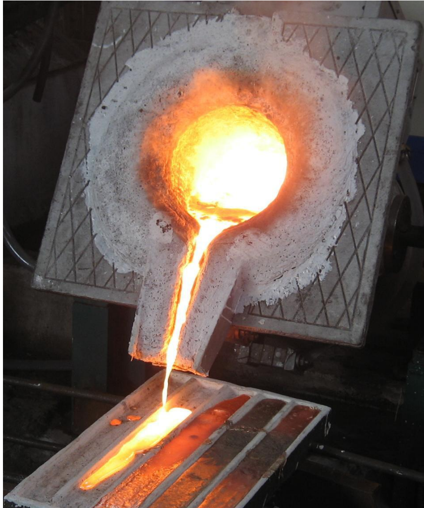
Figure (3.3) below show melting furnace.
