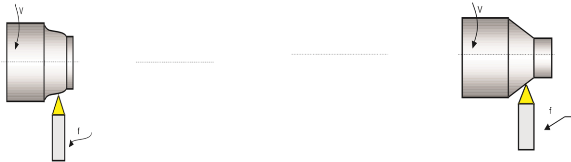
Figure (2.6): Contour turning
