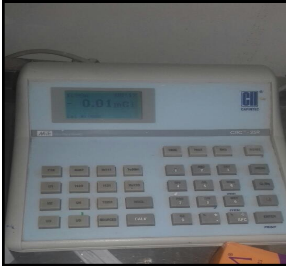
Fig 3.2 shows the display unit of the system consists of display screen with direct reading in Bq or Ci
