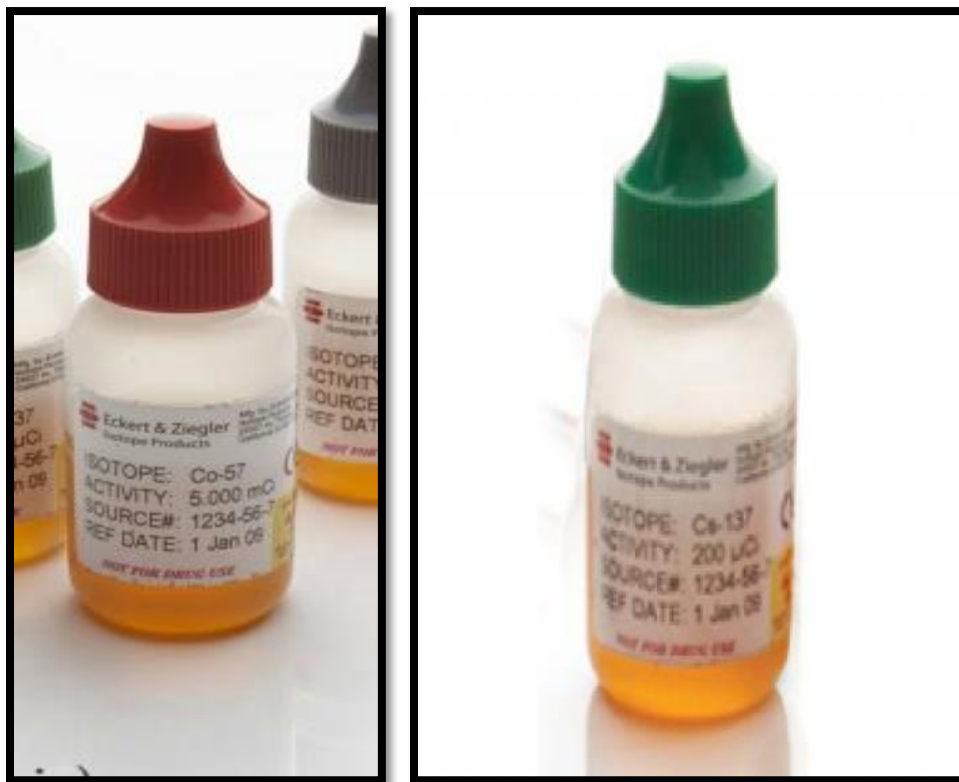
Fig 3.4 shows standard radionuclide source ^{57}\text{Co} and ^{137}\text{Cs} of RICK center.
