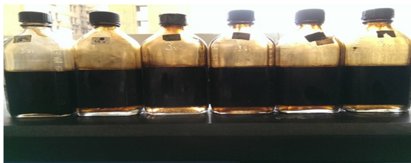
Figure 4 Water separation of OHJ.E20 at five different concentrations at 60°C after 24 hours
