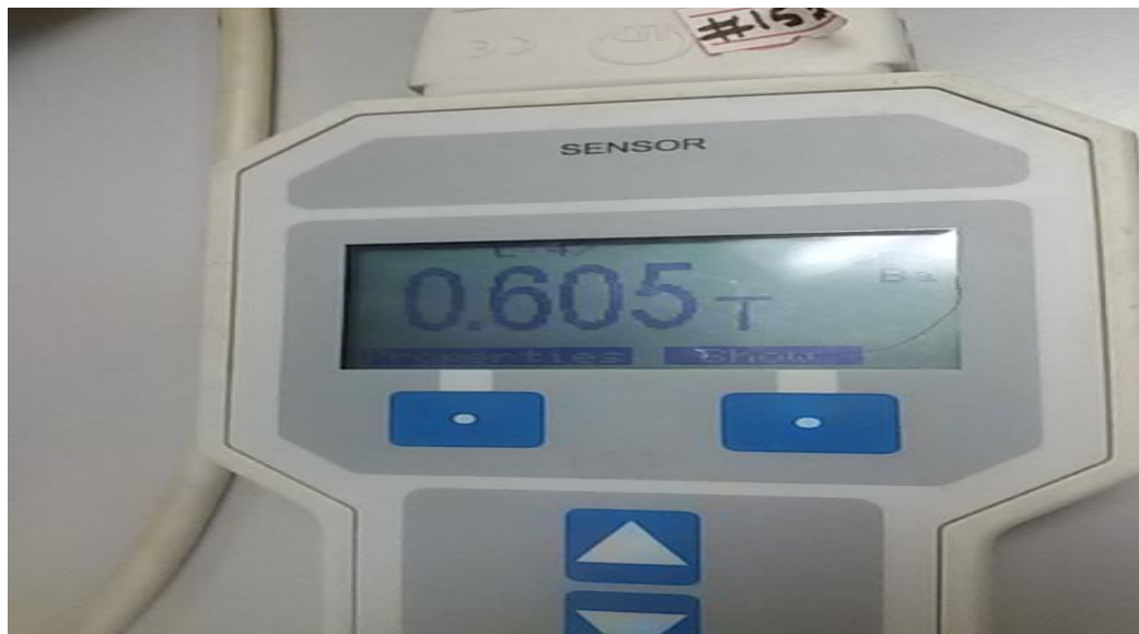
Figure (4-4): 0.6T magnetic field produced by neodymium magnet Nd 2 Fe 14 B measured using teslameter
