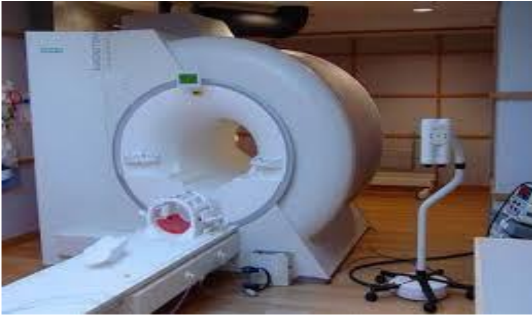
Figure 3.1 :TOSHIBA MRI ( 1.5 tesla) scanner spine array coil used in alzaytona specialized hospital
