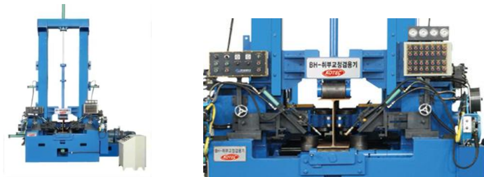
Figure 2.14,15: Integrated system for double purpose - assembling & straightening
