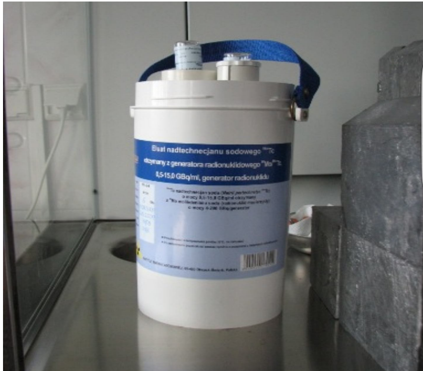
Appendix 3 shows \text{Mo}^{99}\text{-Tc}^{99\text{m}} generator
