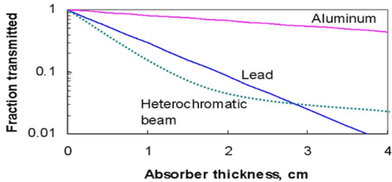
Fig.3.3 Intensity of radiation as function of increasing Thickness
