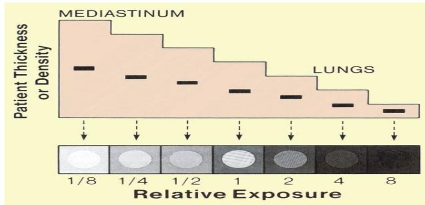
figure .3.5 thickness and relative exposure
