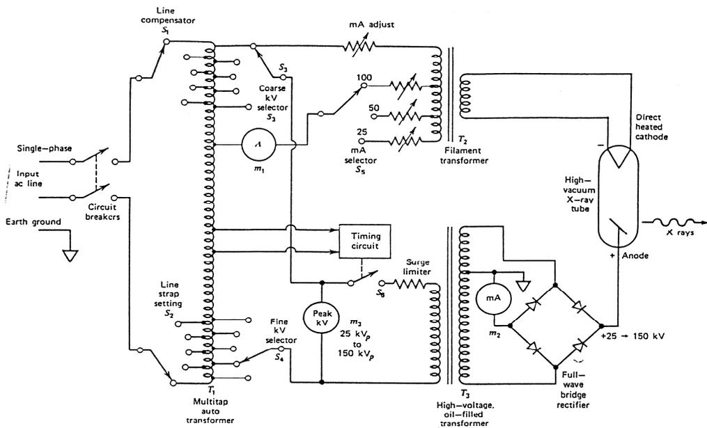
Fig.3.2 Circuit diagram of an X-ray machine.
