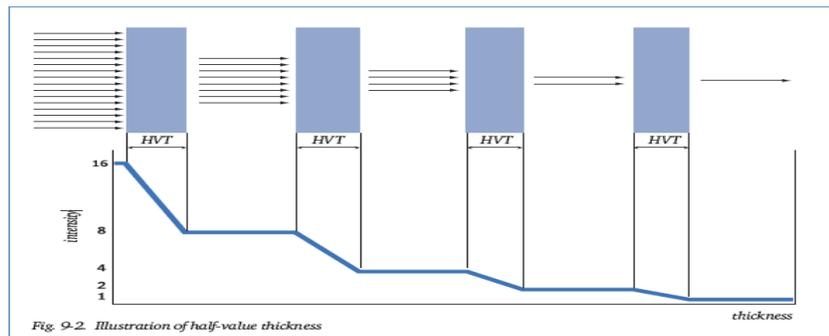
figure .3.4 illustration of half –value thickness
