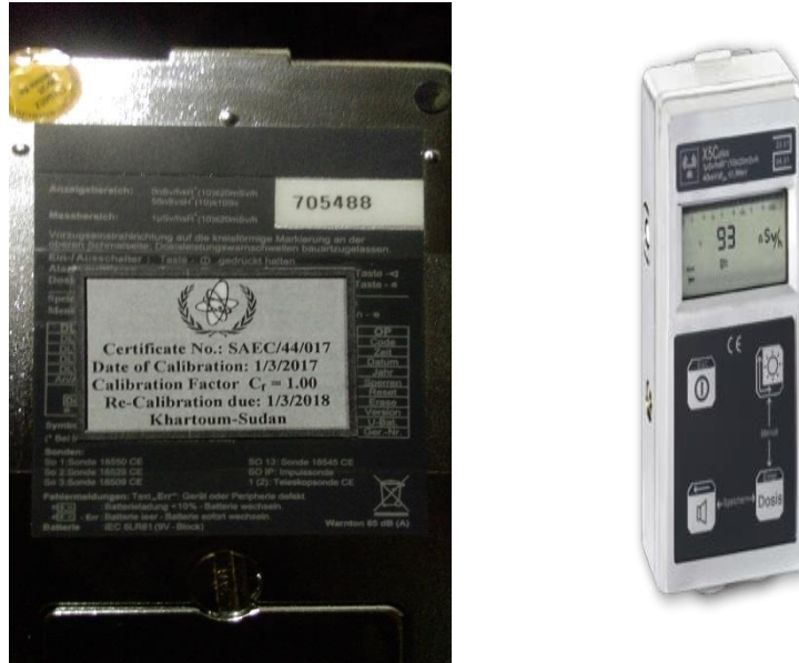
Figure (3.1) shows X5C plus survey meter.
