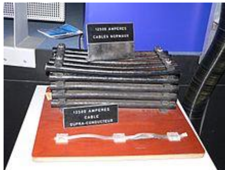
Fig (3.1) Electric cables for accelerators at CERN. Both the massive and slim cables are rated for 12,500 A. Top: conventional cables for LEP; bottom: superconductor-based cables for the LHC
