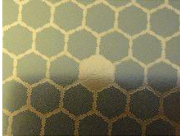
Fig (3.2) Cross section of a preform superconductor rod from abandoned Texas Superconducting Super Collider (SSC).
