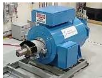
fig(4.9) : motor made with superconductor wire
