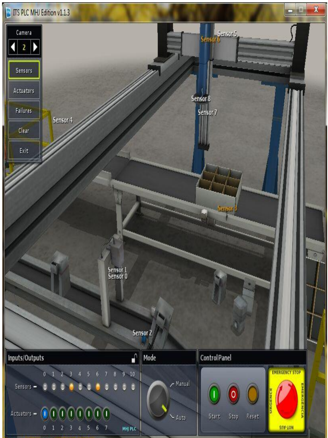
Figure 4-6b: passing of the part conveyor incase wrong part
