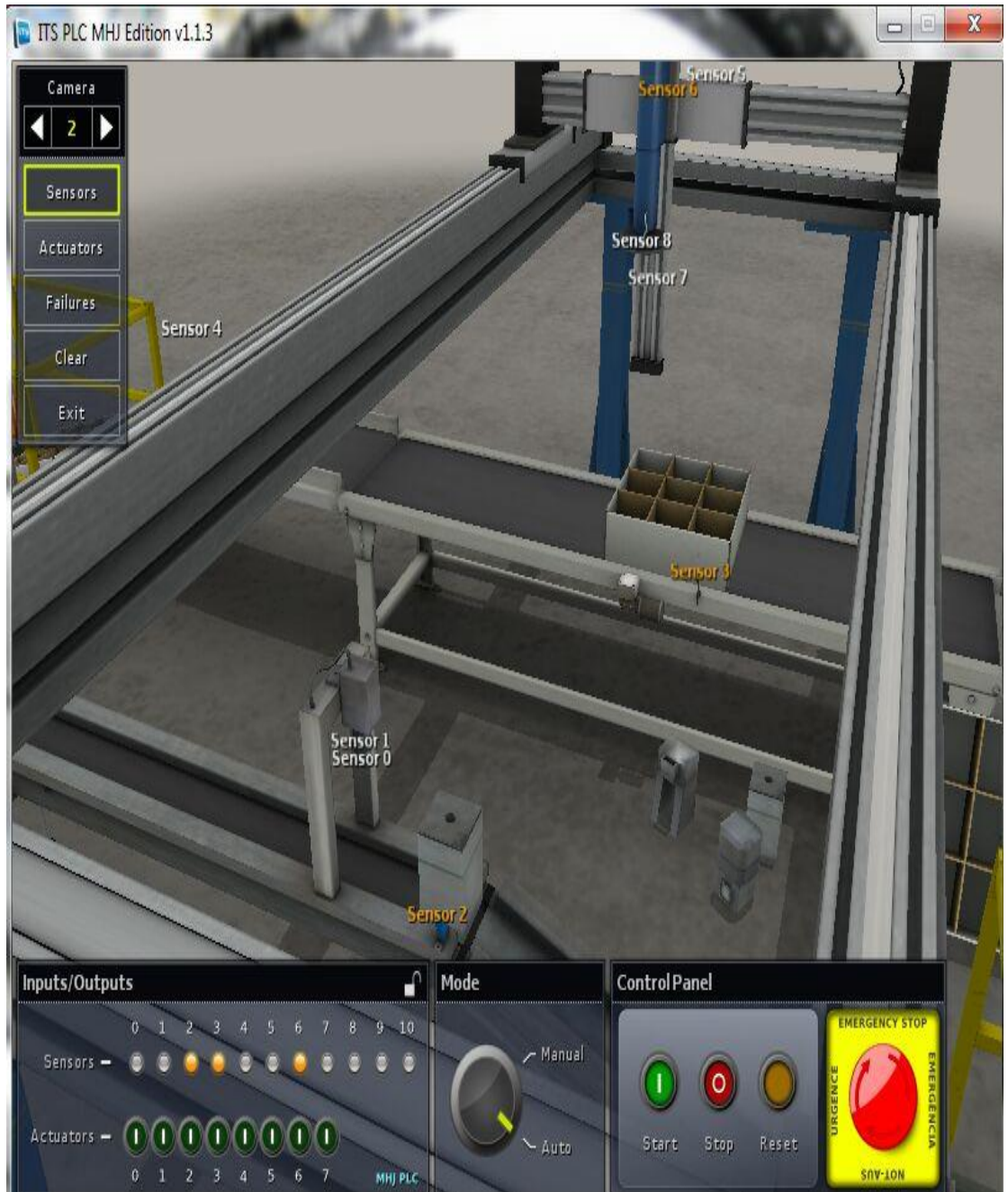
Figure 4-6a: stopping of the part conveyor incase agood part
